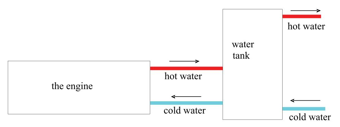
By this way, the heat from the engine is recovered into the water in the water tank. The hot water in the water tank can be used for central heating or sanitary hot water heating. For sanitary hot water, the water tank must be with a coil(heat exchanger) to separate the water from the engine and the sanitary water, to avoid pollution.
