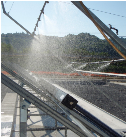
Fig. 3: rain penetration test
